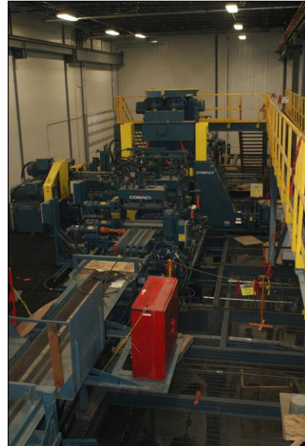
RESOLUTE'S PRODUCTION ASSEMBLY BEING INSTALLED AT ITS SAPAWE PLANT (COURTESY ATIKOKAN PROGRESS)
